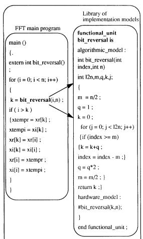
Fig. 2 • Example of an algorithmic/hardware description of a bit reversal operation
