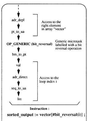
Fig. 5 • Example of implementation of a bit reversal operation with the generic microtask.
